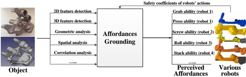
Fig. 1. Schema of using affordances for industrial robotic applications
