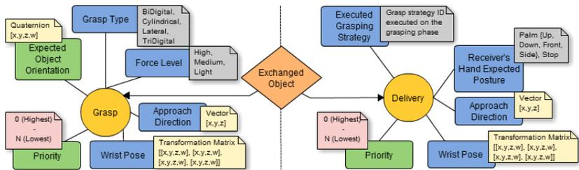
Fig. 2. *Grasp* and *Delivery* model conceptualizations.
